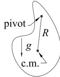
The center of mass is at distance  $R$  from the pivot point. Where is the center of oscillation (*i.e.*, the location of a point mass  $m$  that has the same period as that of the physical pendulum)?
