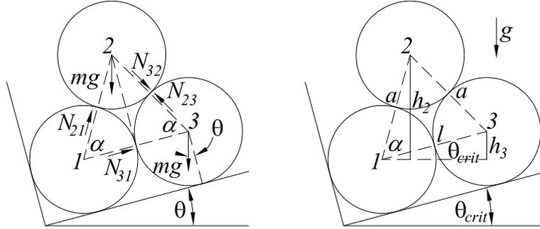
When all the logs touch one another, the forces on log 3 (of mass  $m$ ) parallel to the bed of the truck are related by (ignoring friction),
