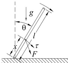
We also consider the torque equation for the upper portion of the chimney (before it breaks), from  $x$  to  $l$ . The center of mass of this segment is accelerating, so we use its center of mass as the reference point. Noting that  $\mathbf{F}$  and  $\boldsymbol{\tau}$  at  $x$  on the upper segment are equal and opposite to those on the lower segment, we have,
