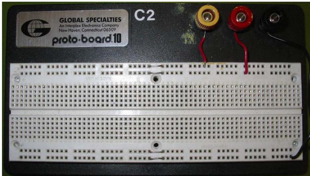
Circuit components can be quickly connected together electrically by pushing their leads into adjacent holes of a connected set. The connections are on the bottom of the board, as shown in the photo below:
