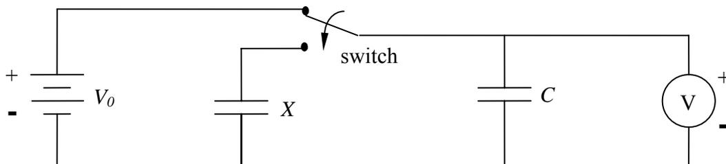
The voltmeter has a large but finite internal resistance. As a consequence the voltmeter discharges the capacitors slowly, which will cause an uncertainty in your determination of capacitance  $X$  if you wait too long to read the voltmeter. Deduce the value of the internal resistance of the voltmeter by observing the time dependence of the voltage across capacitors  $C$  and  $X$ .
