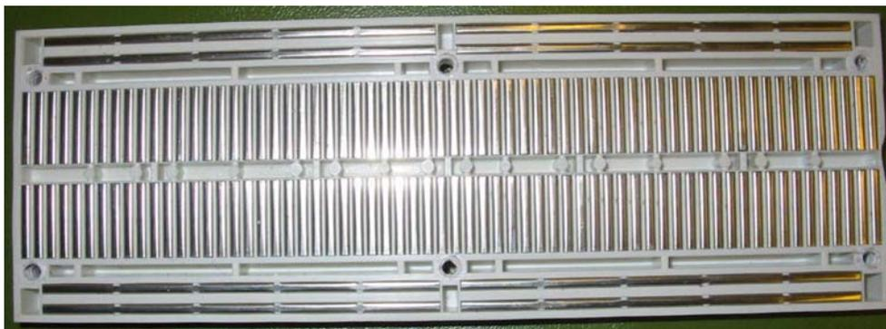
Thus, the entire top row of holes is interconnected, as are the other 3 horizontal rows as well. Similarly, each vertical group of 5 holes is connected together.
