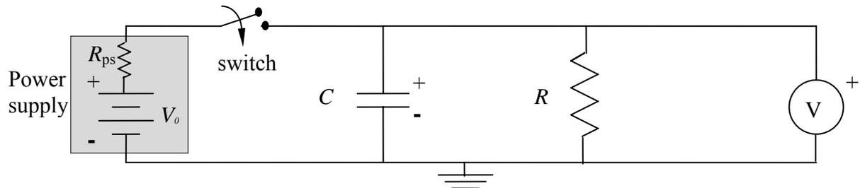
Measure the voltage across the capacitor as a function of time after the switch is opened. (Note: It is not enough merely to switch off the power supply, because the power supply then remains as an element in the circuit.)
