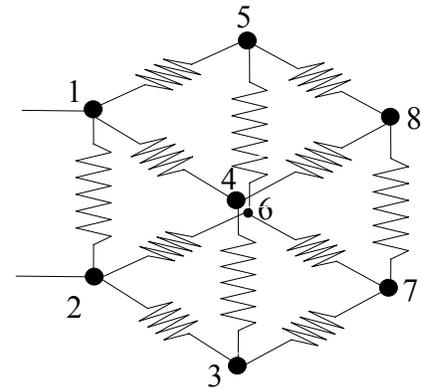
If the leads are connected to points 1 and 3, note that  $V_2 = V_4 = V/2 = V_6 = V_8$ . Thus, resistors 1-2 and 1-4 are in parallel and can be replaced by a single resistor of value  $R/2$ . Likewise, 2-3 and 3-4 merge into one with  $R/2$ , 5-6 and 5-8 merge into one with  $R/2$ , and 6-7 and 7-8 merge into one with  $R/2$ . Now it is "straightforward" to finish the analysis.
