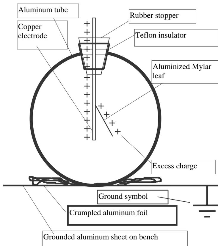
*By “grounding” a conductor, you permit charge to flow between it and the Earth until they are both at the same electric potential (voltage). Because the planet Earth is large compared to the*
