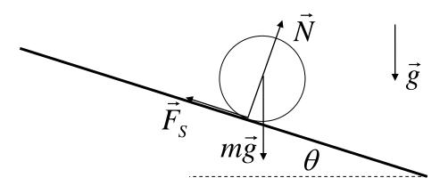
Before we investigate the laboratory setup, let's first consider a simpler problem consisting of a single wheel of mass m, radius r, and moment of inertia  $I = \frac{1}{2}mr^2$  rolling up a ramp inclined at angle  $\theta$  to the horizontal. The wheel **rolls without slipping**, which requires there to be a nonzero force of **static friction**  $F_s$  as it slows down while moving up the ramp. Ignore **rolling friction** for parts a and b below.
