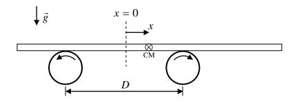
Now suppose that the disks rotate in the opposite direction, so that the one on the right is rotating clockwise and the one on the left counterclockwise.
