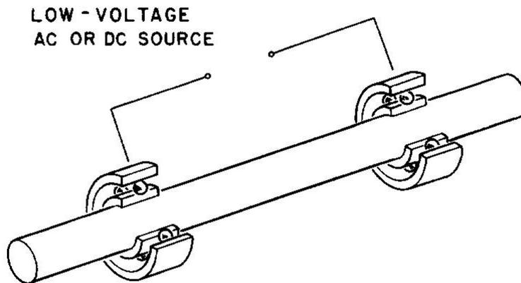
The motor can start from rest (although not all observers report this [1]-[24]), and rotates in either sense, if the current (AC or DC!) is large enough.
