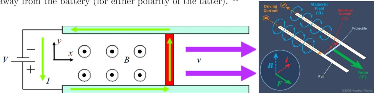
In these experiments with sliding contacts, the current density (for a given total current) at the sliding contact is not as large as that in experiments with a rolling contact, and the Lorentz-force explanation is largely satisfactory.<sup>14</sup>
