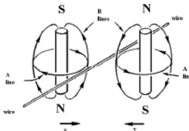
In any quasistatic configuration, the conducting wire would be an equipotential, with zero potential difference between its two ends. This includes the case that the two magnets move towards, or away from, the wire, always keeping the same distance from it, during which motion the magnetic field along the wire is always zero. However, if one measures the voltage difference between the ends of the wire during the above motion of the two magnets, a nonzero result is observed.
