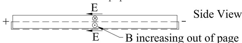
In particular, consider the loop shown by the dashed box in the sketch above, which is in a "vertical" plane that includes the axis of the wire. This loop is "below" the axis of the wire, and the magnetic field is out of the page there. As the two permanent magnets approach one another as in the figure on p. 1, the magnetic flux through the loop increases, which leads to the electric field  $\mathbf{E}$  to the "left" as shown at the "bottom" of the wire.
