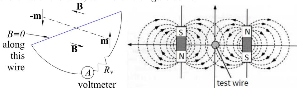
The loop consisting of the (blue) wire and the voltmeter has nonzero magnetic flux  $\Phi = \int \mathbf{B} \cdot d\mathbf{A}$  through it, which increases when the two magnetic dipoles  $\mathbf{m}$  and  $-\mathbf{m}$
