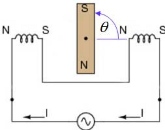
The magnetic field due to the solenoid can be approximated as uniform over the (rotating) permanent magnet.<sup>1</sup>
