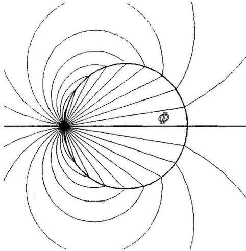
Inside the circuit the equipotentials are straight lines that emanate from the battery. Outside the circuit the equipotentials are circles that pass through the battery. The corresponding electric field lines are shown below.
