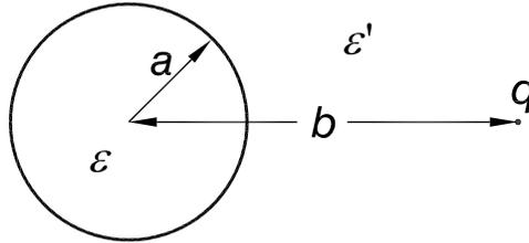
In this three-dimensional problem we take the center of the sphere to be the origin, and take the position of the point charge to be  $(r, \theta, \phi) = (b, 0, 0)$  in a spherical coordinate system. The geometry is azimuthally symmetric, so the potential does not depend on coordinate  $\phi$ .
