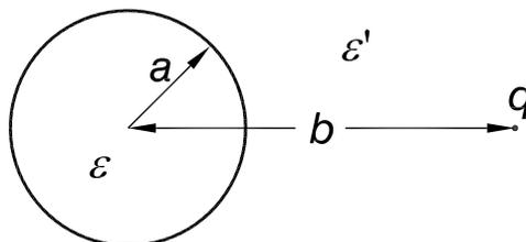
In this two-dimensional problem we take the axis of the cylinder to be  $z$  axis, and the position of the wire to be  $(r, \theta) = (b, 0)$  in a cylindrical coordinate system  $(r, \theta, z)$ . Then, the
