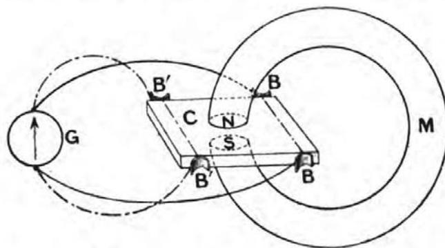
In 1915, p. 559 of [2], Hering described a variant of the experiment sketched on the right above, in which the field of the permanent magnet was perpendicular to a fixed copper plate in the magnet gap, connected to a galvanometer by sliding contacts that were moved from inside of the magnet to outside.<sup>1</sup>
