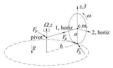
Rolling friction  $\mathbf{F}_R$  has only a 2-component, while static (or sliding) friction  $\mathbf{F}_S$  and the pivot force  $\mathbf{F}_P$  can point in any direction. For now, we suppose that  $F_{P1}$  could be nonzero.
