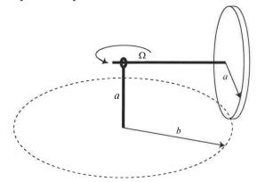
The motion is steady, with constant angular velocity  $\Omega$  about the vertical, assuming no dynamic friction due to air resistance or rolling friction at the ground or at the bearings on the axle.
