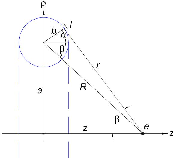
Cullwick noted [7] that the relation (4) has the same form as Maxwell's equation for the magnetic field due to a conducting wire that forms a (solid) torus of the same dimensions as the (hollow) toroidal magnet when the wire carries azimuthal current density  $\mathbf{J} = J \hat{\phi}$ ,
