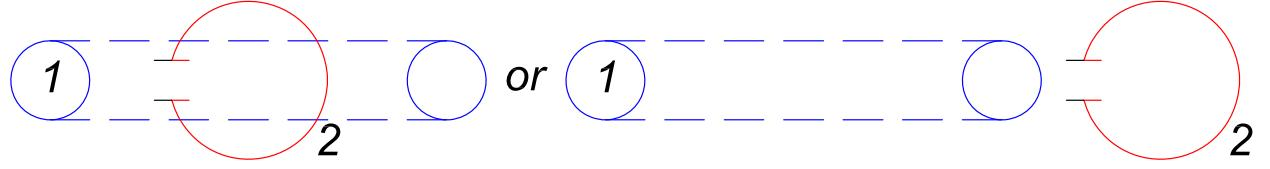
The  $\mathcal{EMF}$   $\mathcal{E}_1$  induced in the toroid by an oscillatory current  $I_2 e^{i\omega t}$  in the  $LC$  circuit is,
