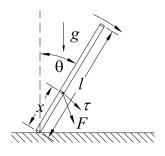
We also consider the torque equation for the upper portion of the chimney from x to l (before it breaks). All points on this segment are accelerating, so it is perhaps best to use its center of mass as the reference point. Noting that  $\mathbf{F}$  and  $\boldsymbol{\tau}$  at x on the lower end of the upper segment are equal and opposite to those on the upper end of the lower segment, we have,
