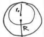
$$\text{APOGEE IS } 2R - r_0 = r_0 \left( 1 + 4 \frac{V_x}{V_i} \right) \quad V_i = r_0 \Omega$$
