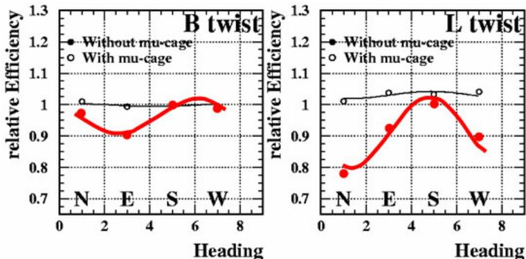
The suppression of the magnetic field by the wire-mesh shield is not fully effective at radii within about one mesh spacing of the mesh itself, and indicated in the figure below (from [16]).
