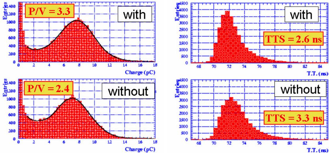
These effects are not large, so that many experiments, including LSND [7], and mini-BooNE [8] and the Pierre Auger Project [9], operate large PMTs with no magnetic shielding (since the classic technique of shielding a PMT with a  $\mu$ -metal cylinder is awkward for large PMTs in tanks of liquids). Other experiments, including Super-Kamiokande [10], SNO [11], KamLAND [12] and BOREXINO [13], surround the entire detector with field-compensating coils to cancel some components of the Earth's field.
