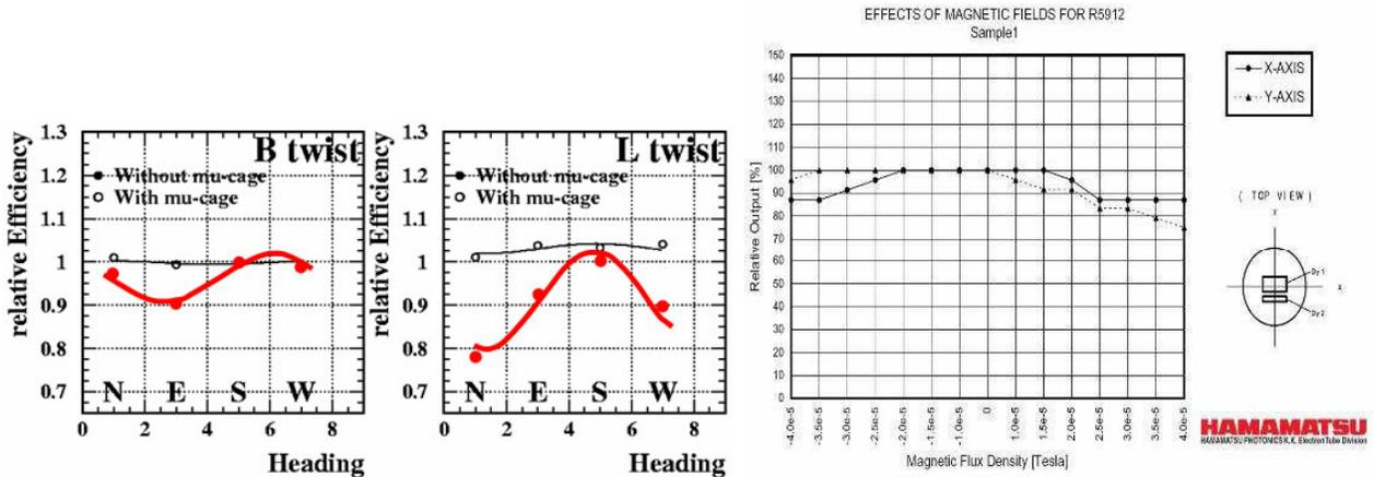
Note that the gain of a well-designed PMT such as the Hamamatsu R5912 is largely unaffected by magnetic fields large than  $\approx 1/3$  of the Earth's field, as shown in the figure on the right above.
