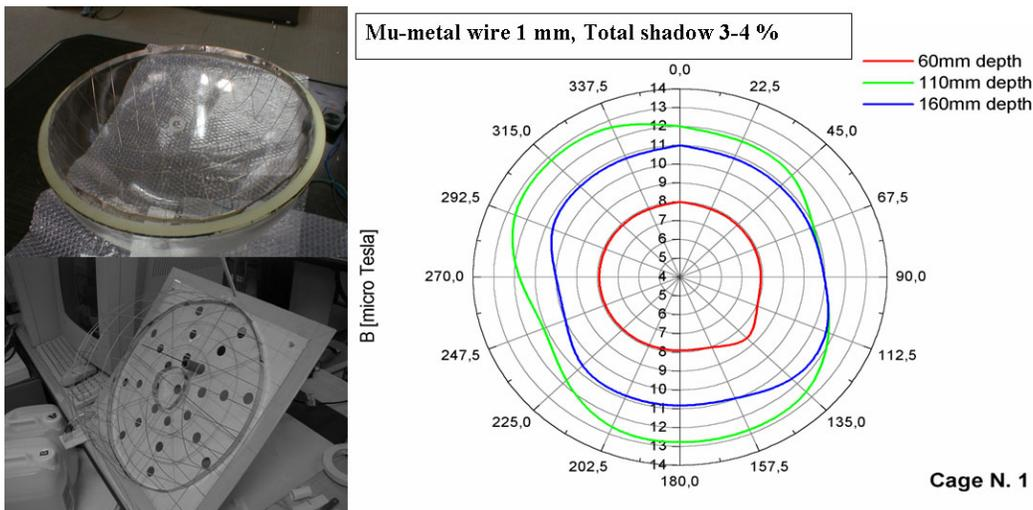
In the Appendix we deduce that a solid shell of high permeability  $\mu$ , radius  $a$  and thickness  $\delta a \ll a$  provides a shielding factor of,
