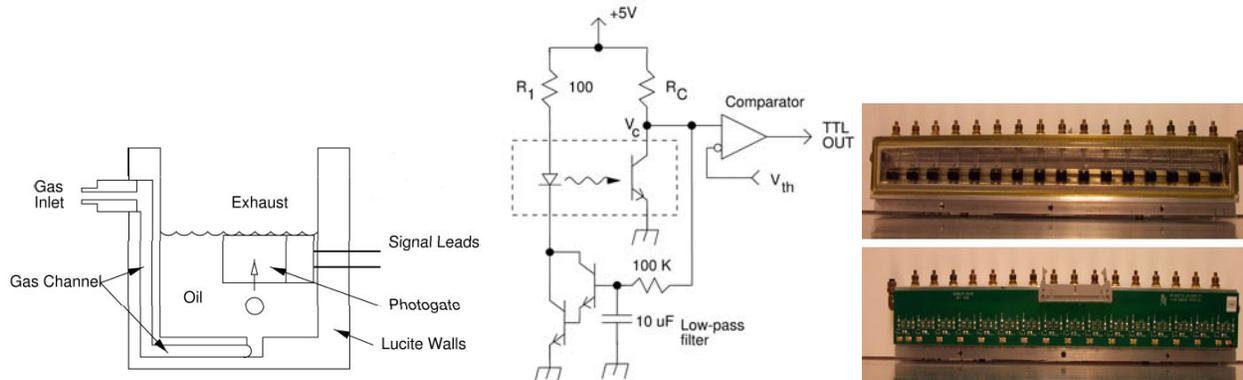
Fig. 0.3. Concept, circuit diagram and photographs of the electron bubbler system. From[3].
