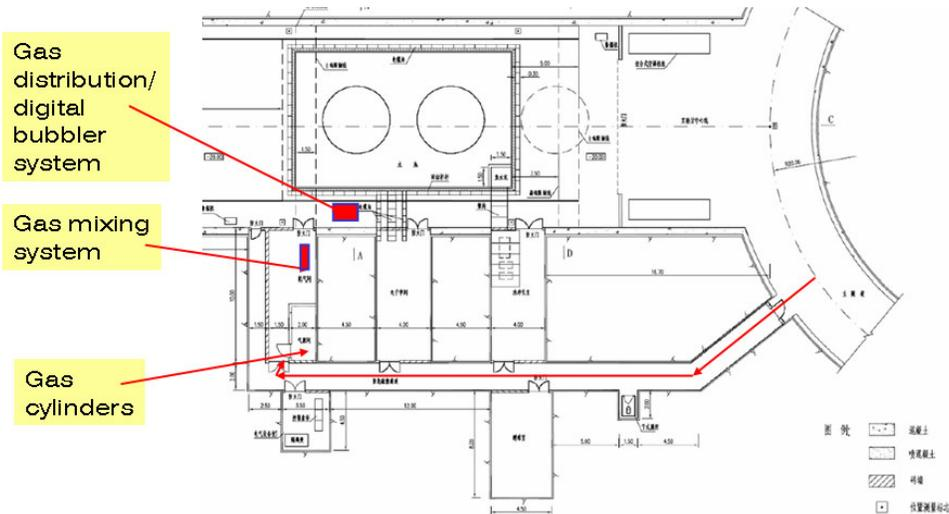
Fig. 0.5. Layout of the RPC gas system in one of the Near Halls.
