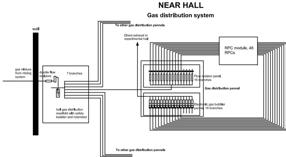
Fig. 0.1. Overall process diagram of the RPC gas system in one of the Near Halls. From[9].
