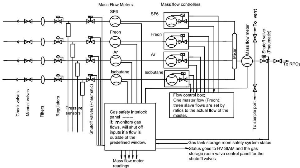
Fig. 0.2. Process diagram for the gas mixing subsystem. From[9].
