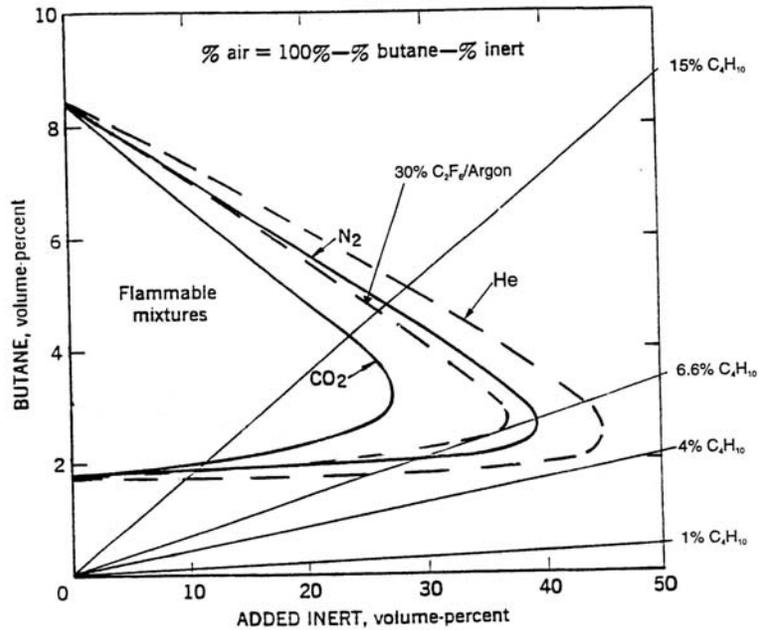
Fig. 0.4. Flammability regions for isobutane gas mixtures. There is no region of flammability for a gas mixture in which the ratio of isobutane to the inert component of the RPC gas is 4% or less. From[10].
