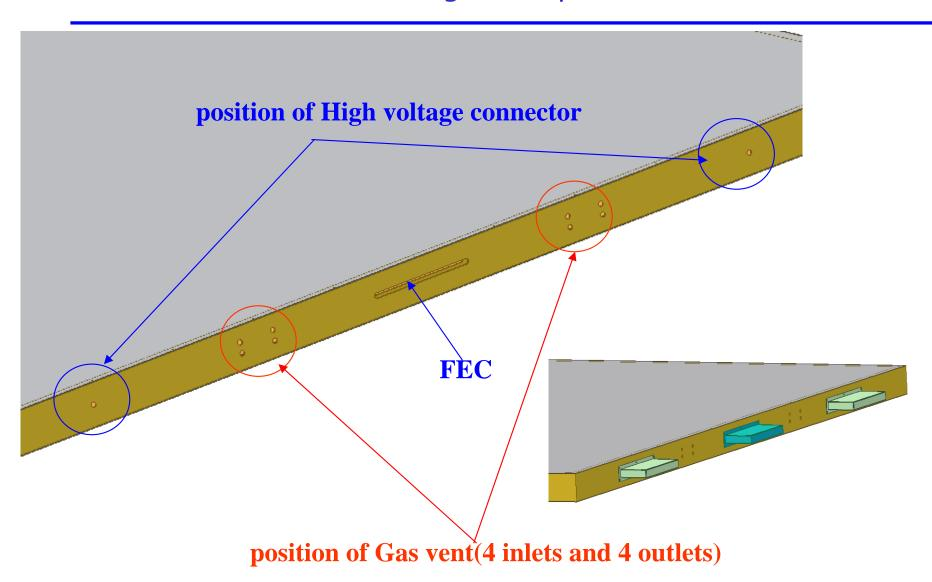
Proposed layout is fine, assuming that the FEC boxes and HV interface boxes provide electrical shielding.
