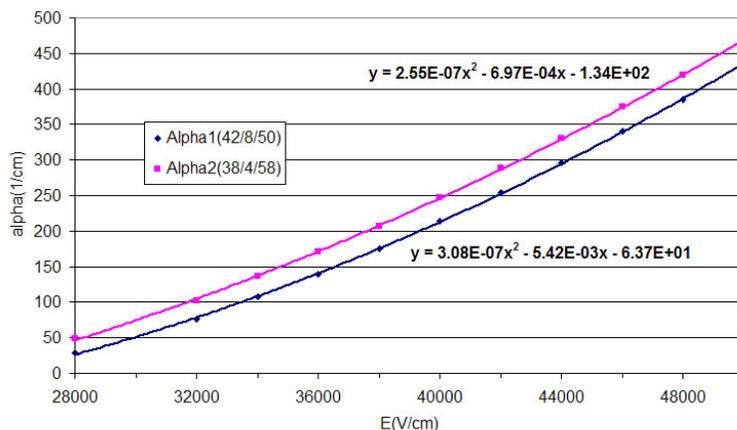
Figure 3: Townsend coefficient for two RPC gas mixtures, Freon/Isobutane/Argon: 42/8/50 and 38/4/58 at 1 atmosphere pressure, calculated using the MAGBOLTZ program [1].
