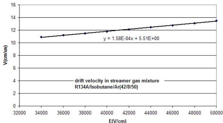
Figure 2: Drift velocity in the RPC gas mixture Freon/Isobutane/Argon: 42/8/50 at 1 atmosphere pressure, calculated using the MAGBOLTZ program [1].
