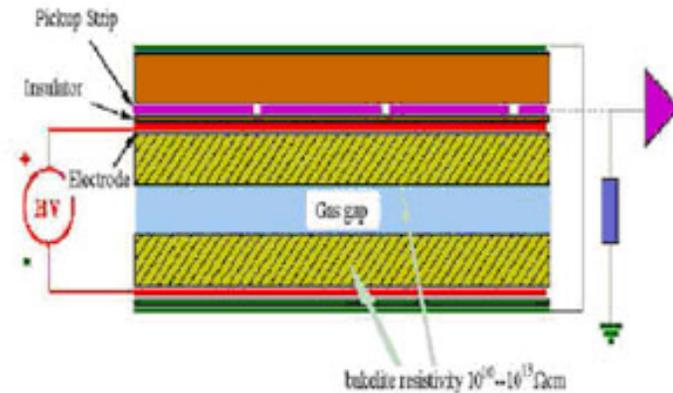
Figure 1: Sketch of a Resistive Plate Chamber (RPC).
