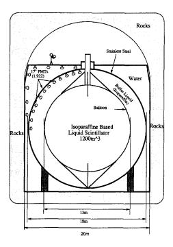
Figure 2. Schematic view of the KamLAND detector.
