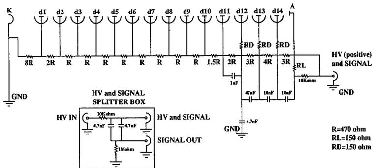
Fig. 1. The HV divider and the signal splitter box for the EMI 9356KA photomultiplier.
