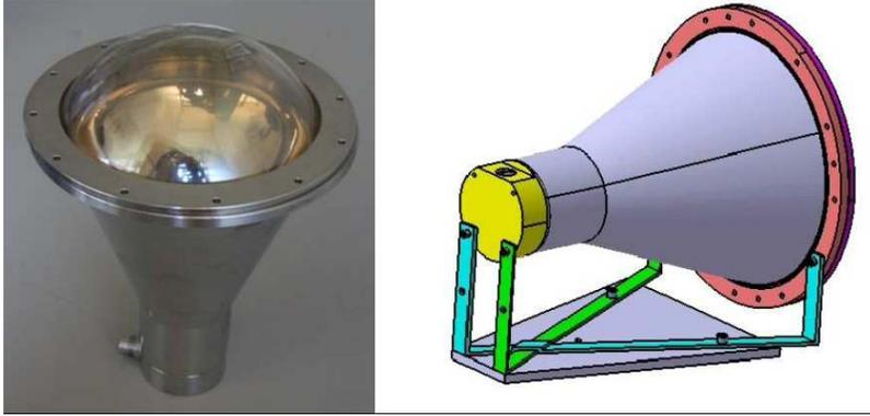
Figure 56: PMT encapsulation and mounting (Drawing P. Guillouët)
