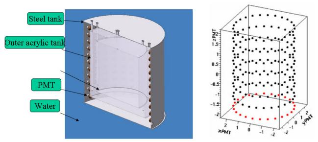
We label the PMTs by the index i which runs from 1 to N = 224. The number of photoelectrons observed (during some appropriately narrow time window) in PMT i is denoted  $n_i$ , and the "gain" of PMT i in units of MeV per photoelectron is  $G_i$ .<sup>1</sup> The signal S in MeV from a scintillation process such as neutron capture is,
