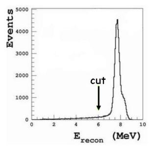
The strongest requirement on the calibration of the scintillation process is that the energy scale at 6 MeV be known to an accuracy of 1% so that the effect of a cut at this energy on the efficiency of neutron detection is less than 0.2%.
