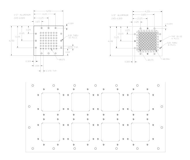
Figure 4.14: Cable feedthrough and mounting panel.
