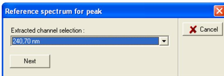
In this screen, select the extracted chromatogram in which the reference spectrum will be associated. Press *next* to display the following screen:
