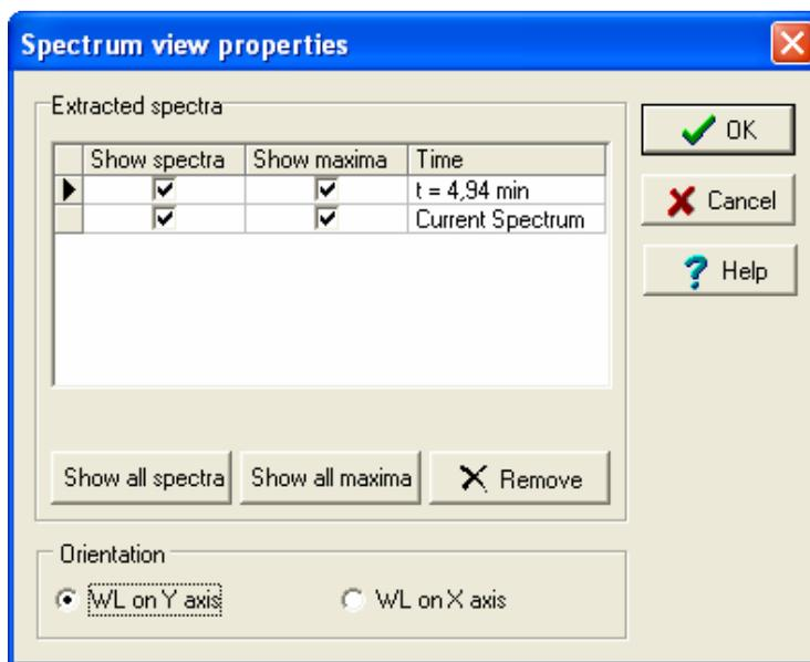
Choose which spectrum(a) you want to display by checking the corresponding box in the *Show spectra* column.
