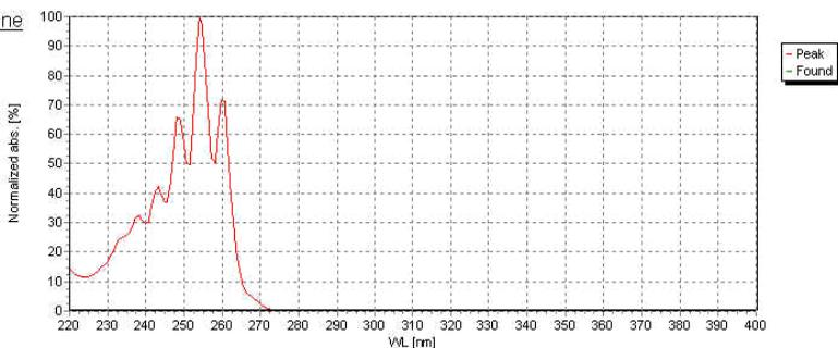
According to the Galaxie Report Editor object properties, the libraries and parameters used for the search can be printed and for an unknown spectrum, the report gives the library spectrum name, its retention time, the matching factor and the library from which it is extracted.
