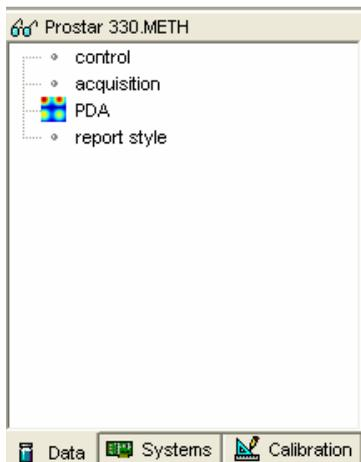
Click on the parts of this method to edit the parameters in the right part of the screen.
