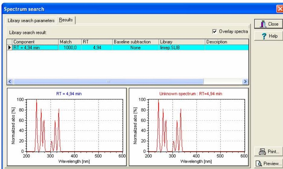
The correlations are calculated and the candidate spectra are displayed in the spectrum table. For an unknown spectrum, the
