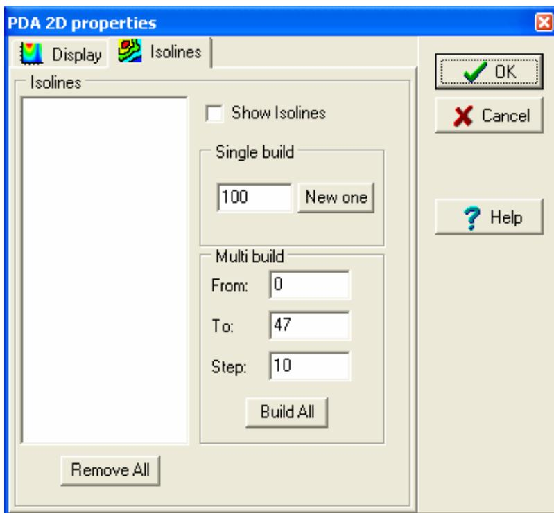
In the **Isoline** tab, check **Show Isolines** if you want to display isolines.
