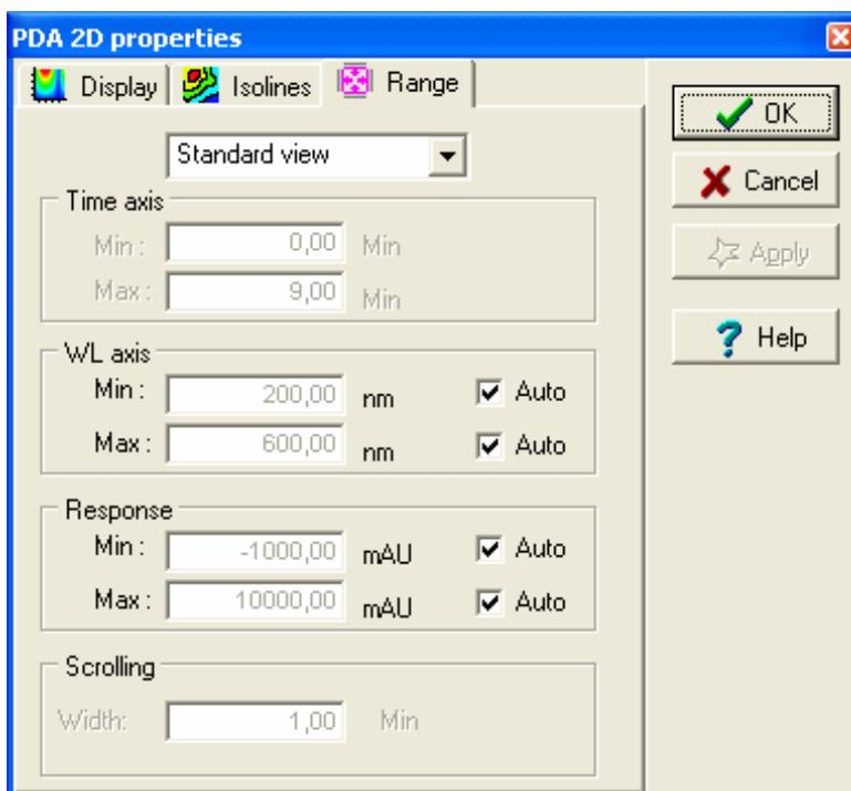
In the **Range** tab, you can choose the acquisition view properties (standard, fixed, or scrolling view) using the scrolling list. If the standard view is chosen, you can modify the Wavelength and the Response axis range. If the fixed view is chosen, moreover, the Time axis range can be modified. If the scrolling view is chosen, the scrolling width must be fixed in the field.
