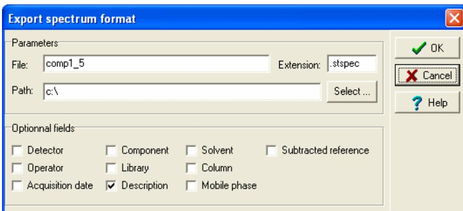
This window is divided into 2 parts, the 'Parameters' of the export and some 'Optional Fields' if a reference spectrum from a library is to be exported and 3 parts if a spectrum from a spectrum view is going to be exported.
