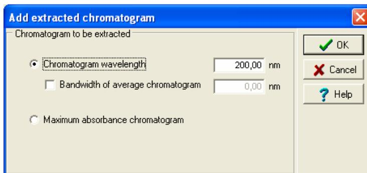
You can choose to extract a chromatogram at either a given wavelength or at an average wavelength over a defined bandwidth, or at the maximum absorbance chromatogram obtained on the full acquisition wavelength range or in a user defined wavelength range.
