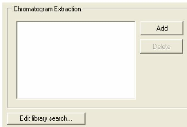
In the Chromatogram Extraction field, you can **add** the chromatogram you want to automatically extract after the acquisition. Click on the *Add* button, to choose the chromatogram you want to extract. The following screen appears:
