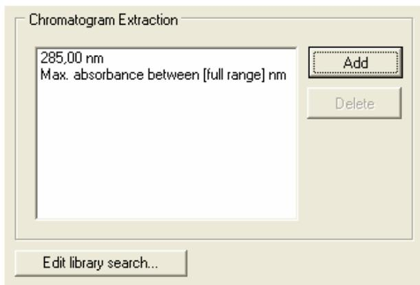
For each extracted chromatogram, a sub-section is created in the browser. Its name corresponds to the wavelength at which the chromatogram is extracted:
