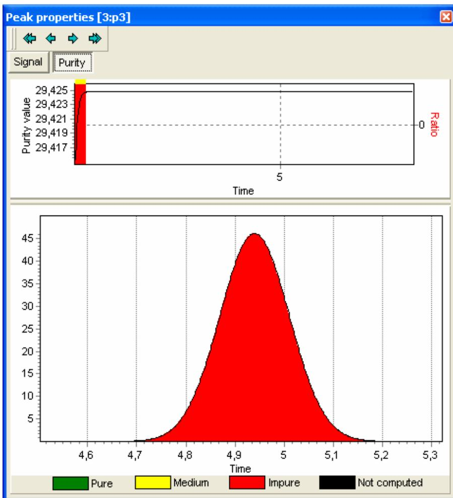
On the top part of the screen, the ratio chromatogram and the purity values are displayed. (A graph relating the variation of the purity versus time is also given for each peak. If ratio chromatograms have been defined, the ratio is also displayed here.).
