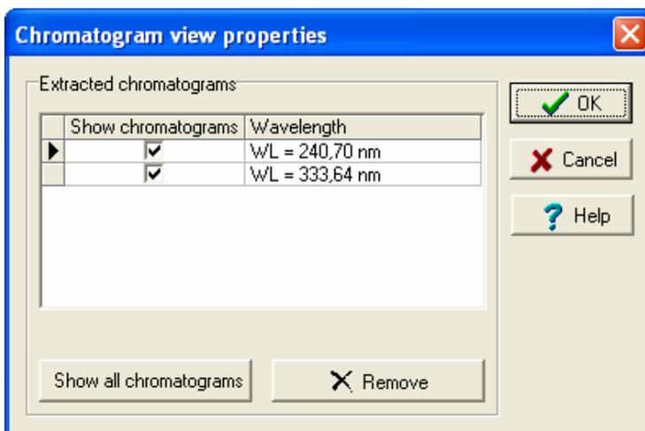
Choose which chromatogram(s) you want to display by checking the corresponding box in the *Show chromatograms* column.
