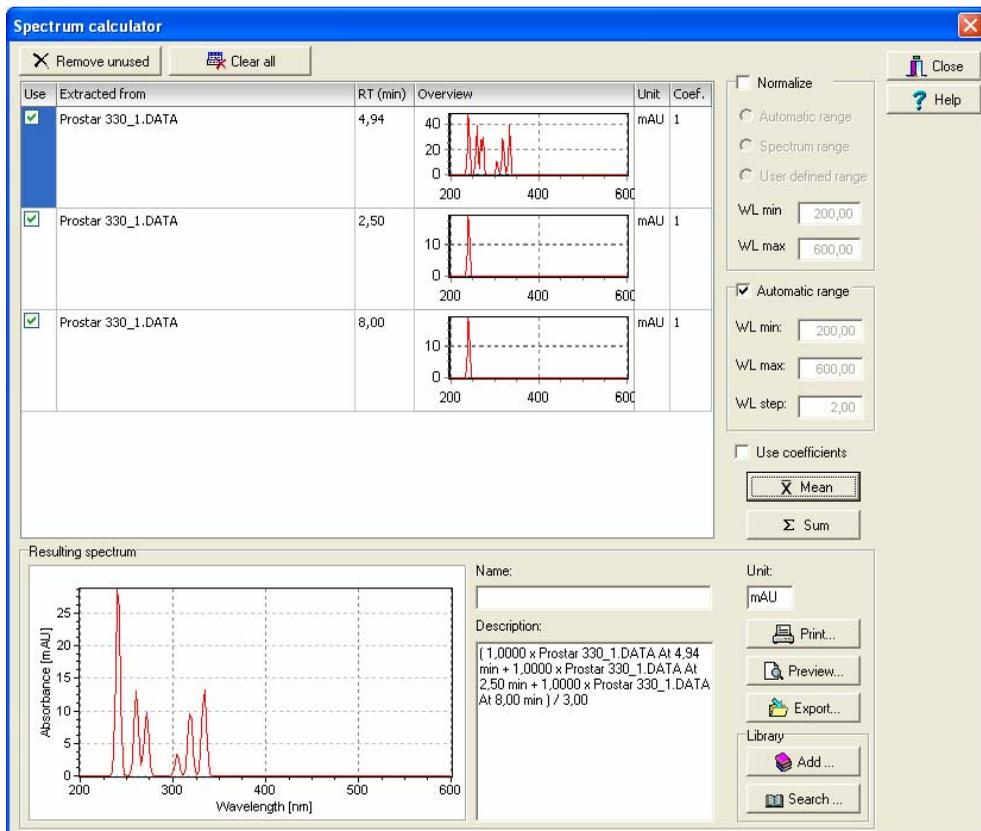
The Spectrum Calculator window is composed of 3 parts: the spectrum list, the parameters settings and the resulting spectrum part.
