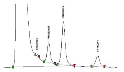
The **tangent skim Next Peaks** event does not work when the mother peak is not fully resolved (e. g. has a valley with the previous peak). The use of a **Baseline Now** event has the effect of removing the valley, and thus allows the skimming event to work properly. See figures below.
