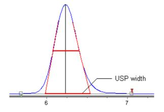
Left Half Width X% [min] [WLX]: Left half peak width measured at the specified height (X). The height is expressed as a percentage of the total height of the peak. 0% of the height is on the baseline, 100% of the height is on the top of the peak:
