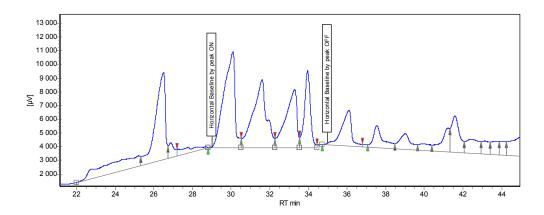
If an event is activated at the beginning of a peak (between the start marker and the peak apex), it becomes operative at the peak start time. If the event is activated at the end of the peak (between the top of the peak and the stop marker), it becomes operative at the peak stop marker time.
