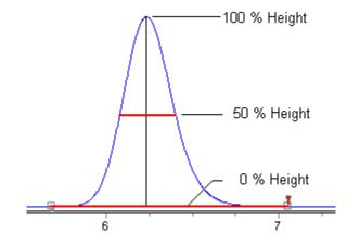
A height of 4.4% corresponds to the 5-sigma method A height of 13.4% corresponds to the 4-sigma method A height of 32.4% corresponds to the 3-sigma method A height of 60.7% corresponds to the 2-sigma method Seven heights are proposed: X= 4 means 4.4 %
