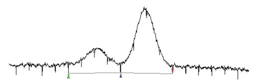
If the spike reduction is activated, the spikes will be eliminated from the signal and the baseline drawn on this signal:
