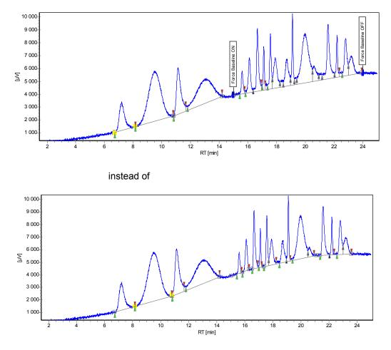
If the forced baseline penetrates the signal, the baseline will automatically adjust so that it always remains under the signal.
