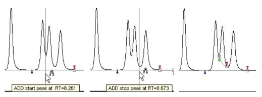
The baseline of shoulder peaks is always a line, either exponential or linear. It is possible to define the shoulder integration mode (tangential or exponential) before moving markers, in the sub menu of the icon:
