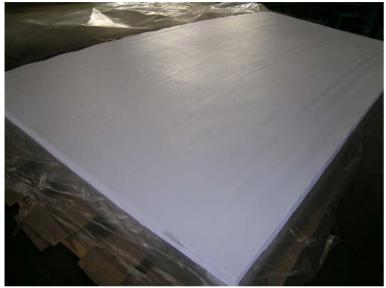
Melamine resin coated and dried brown paper, which is used for the body of Bakelite sheet. Layers of such paper stacked together, sandwiched by two white papers, then placed between two S.S. plates, heated and pressed under 2500 tons pressure.
