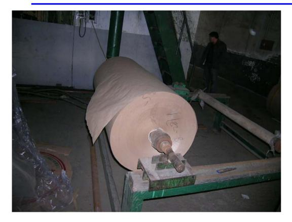
The raw base paper roll is placed at the paper feeding station of the production line, waiting for being fed to resin coating station.
