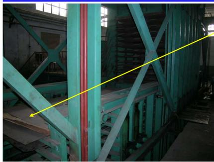
The prepared stack will be inserted into the gap between thick steal blocks, in which hot steam will pass through an embedded hollow channel to heat up the block.
