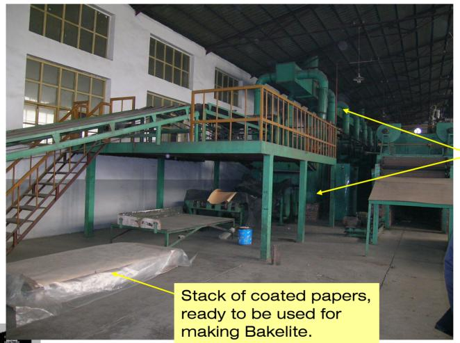
**Resin coating** production line, shown here are two lines – upper and lower, only the lower line is being used for Daya Bay Bakelite production.
