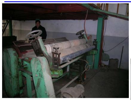
The coated and dried paper will be rolled out from this port, and cut to specified length.
