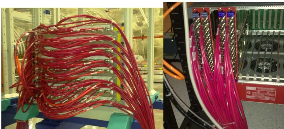
**Fig. 7** pictures of HV (back side of Main Frame and fan-outs)
