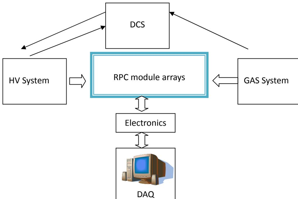
**Fig. 1** schematic diagram of RPC detector
