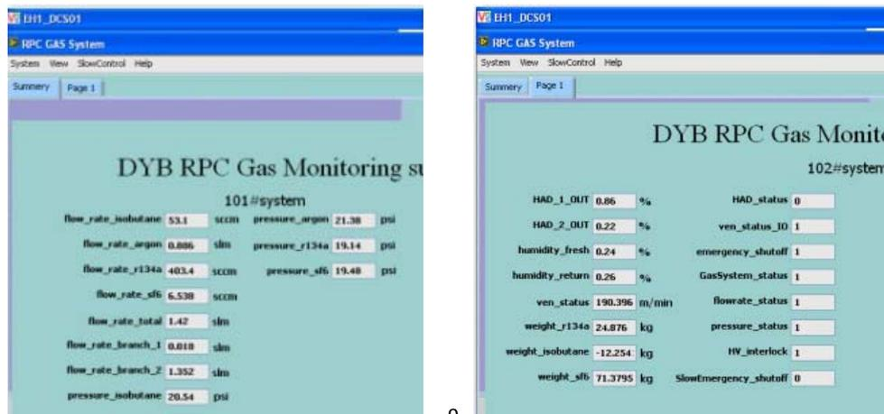
**Fig. 5 Two pages of DCS RPC gas monitoring system.**
