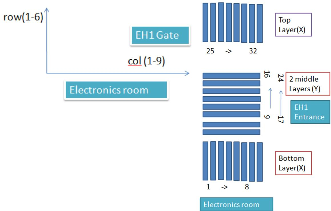
**Fig. 3 coordinate system of RPC module array**
