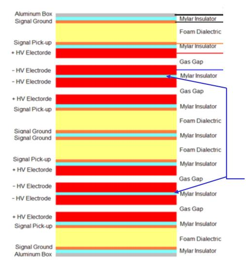
• This RPC module won't work: the polarities in two gaps of one pair RPCs are opposite, so the induced signals seen by the pickup strip from two gaps will cancel each other, strip will get no signal!
