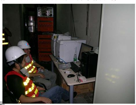
Luo Xiaolan and Xu Jilei are using the GC to analyze the gas sample from AD (see next page for the test result).
