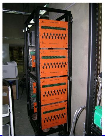
All 7 sets of gas distribution/digital bubblers crates are mounted on one rack as shown on left. Filled with silicon oil, all channels are bubbling. When AD's white oil arrives we'll replace the present silicon oil with the white oil to reduce the viscosity, thus to improve the quality of the bubble.
