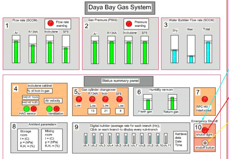
All meters and indicators on screen are passive but this Emergency Shutoff Block.
