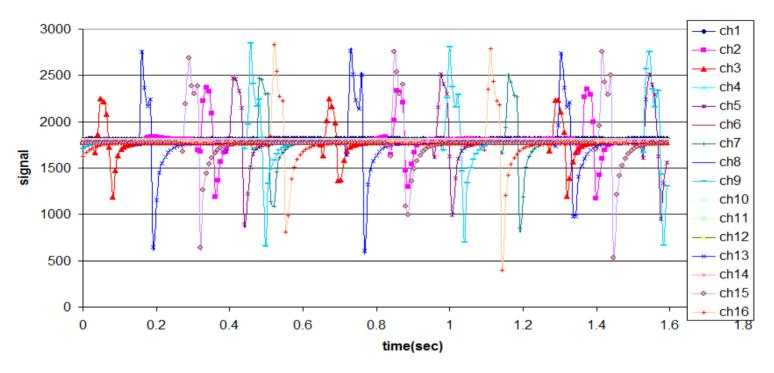
Microprocessor ADC can reconstruct the bubble shape, the digital bubbler system can count the pulse rate and store the data file in a database.
