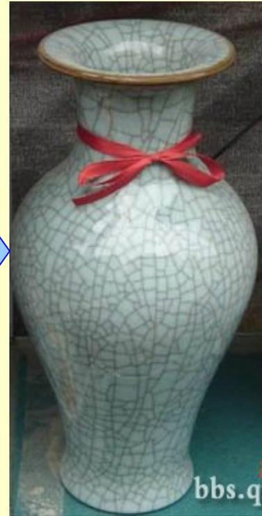
The crackle glaze was the result of the inconsistent thermal expansion coefficient between the body and glaze.
