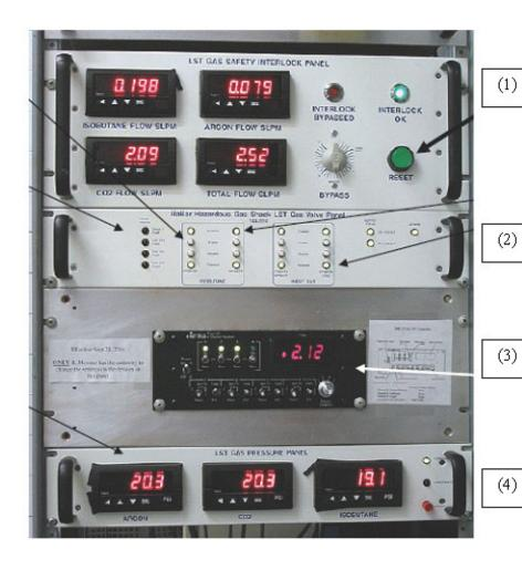
Gas Safety Interlock Panel: displays flow rates and interlock status.
