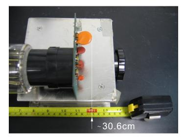
The above 2 pictures show a current workable PMT, which means a PMT itself equipped with base, socket and voltage divider. We will definitely have not enough space (pls refer to the attached pages).
