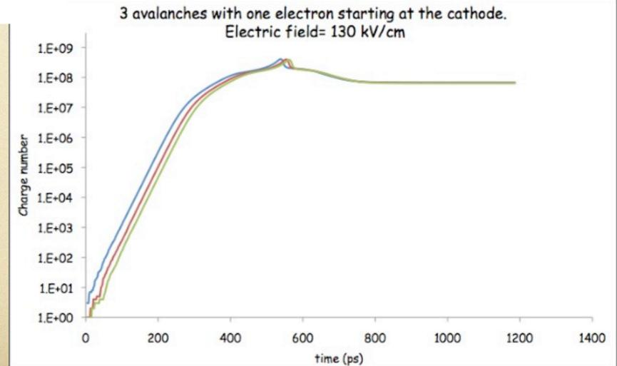
So easy to see that time jitter depends on  $\lambda$  and the time to move  $1\lambda$  (i.e. 1/drift velocity)
