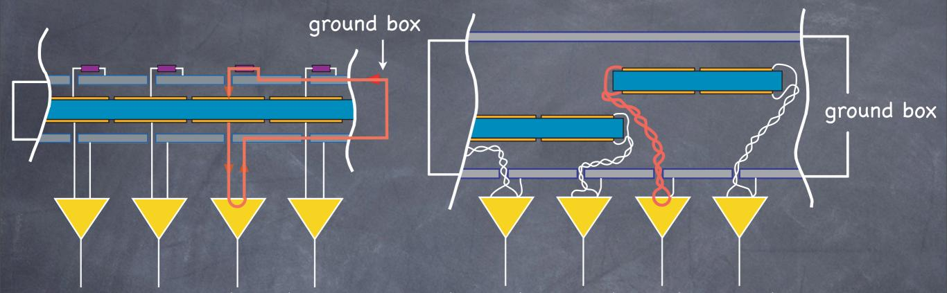
The signal is induced on the anode and cathode pickup pads - current flows from anode pad through amplifier and returns to cathode pad. The strip design allows the use of a transmission line (twisted pair cable) to connect this 'signal generator' to the amplifier - otherwise return path is via the outside grounding box (therefore sensitive to all the noise in the ground). In reality this is a key ingredient to substantially reducing the noise and improving the time resolution
