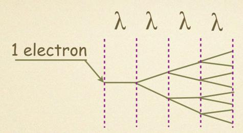
For a given electric field an electron will undergo an ionising collision average every distance,  $\lambda$  , that it travels where  $\lambda$  is the distance between
