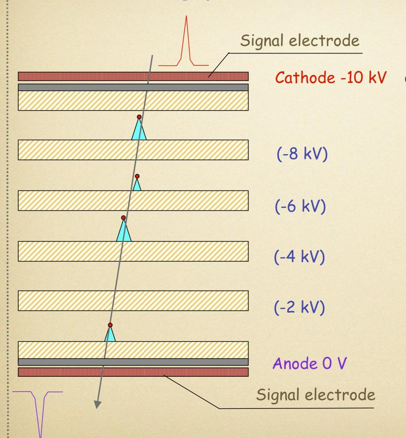
Stack of equally-spaced resistive plates with voltage applied to external surfaces (all internal plates electrically floating)
