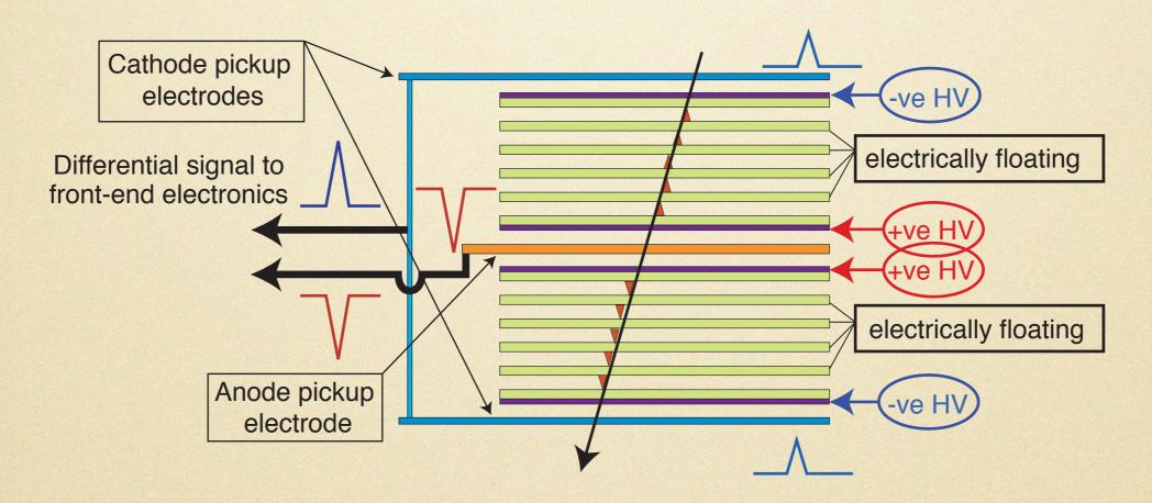
Note: HV only applied to outer surfaces of each stack of glass (internal glass sheets electrically floating) this makes it very easy to build.
