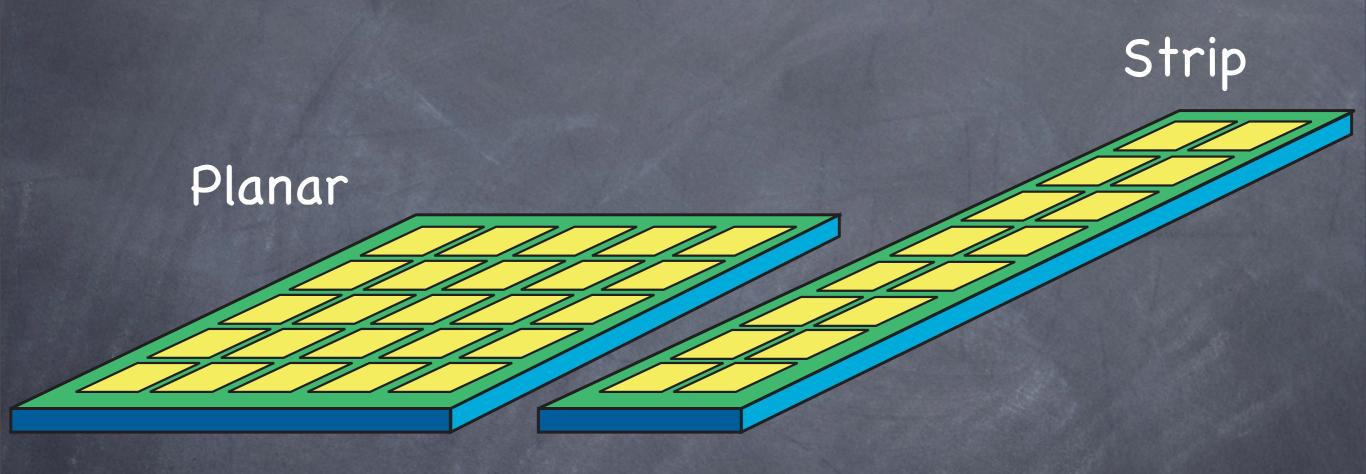
Strip has some advantages concerning the geometry but very large advantage for the readout electronics
