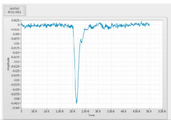
August 24, 2012 APD timimg jitter on Agilent DSO91304A 13 GHz oscilloscope
