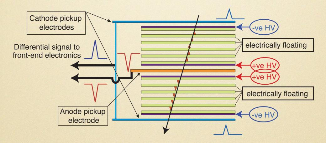
Note: HV only applied to outer surfaces of each stack of glass (internal glass sheets electrically floating) this makes it very easy to build.
