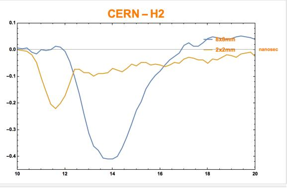
In order not to degrade the signal, preamp and scope bandwidth should be greater than the 300 MHz corresponding to this bandwidth. According to Shannon-Nyquist a sampling frequency of >1-2 GSa/s should be adequate.
