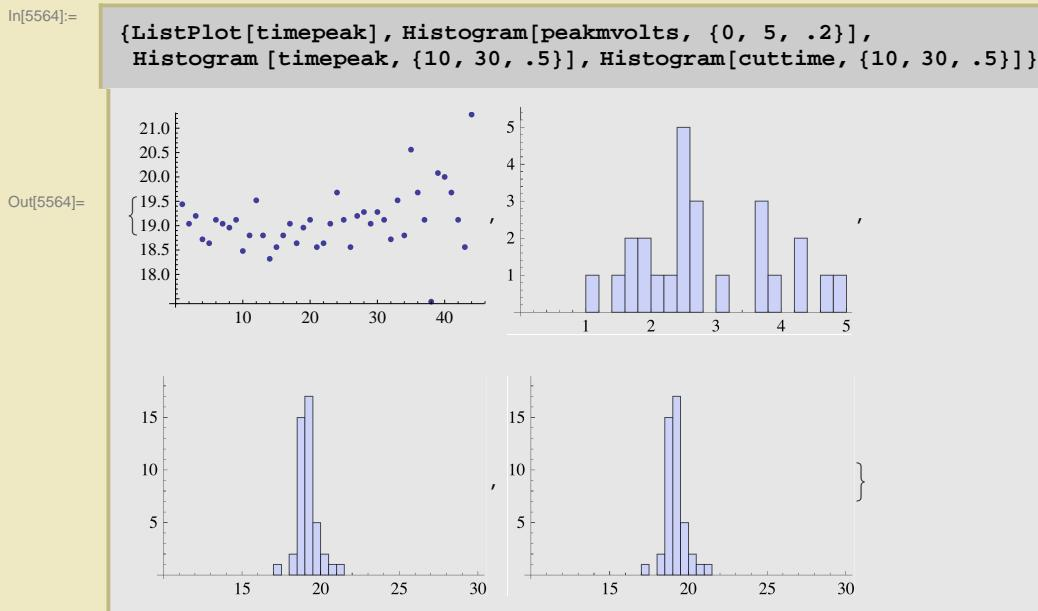
**Calculate Speed of Electron. A couple problems with this are pileup at the 20 cm position and crudeness of using peak channel for time.**
