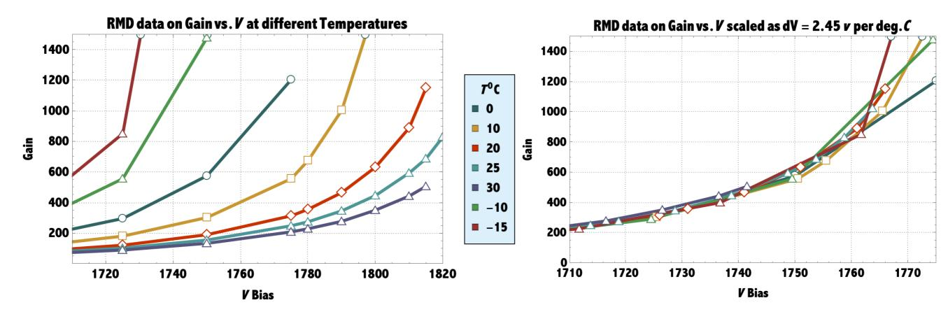
RMD 8x8mm<sup>2</sup> avalanche diode Gain vs. bias voltage response for 20 nsec(wide ?) 425nm laser pulses. Unity gain refers to the amplitude obtained at the ~300V bias where amplitude is roughly V independent.
