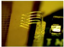
8x8mm<sup>2</sup> Silicon Sensor capacitive readout woven MMegas mesh replaced by eForm Ni
