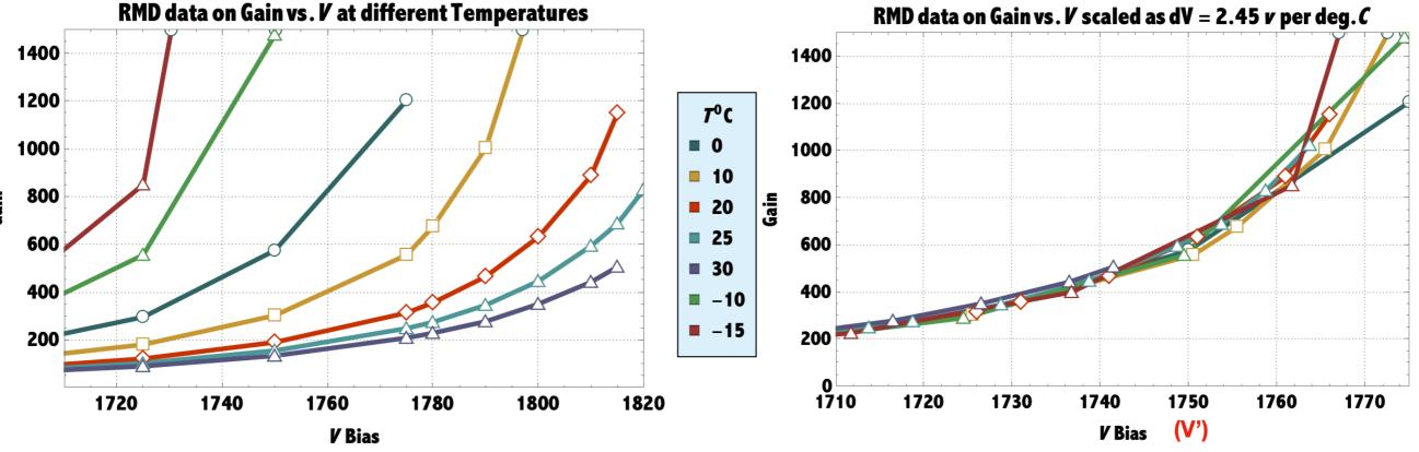
RMD 8x8mm<sup>2</sup> avalanche diode Gain vs. bias voltage response for 20 nsec(wide ?) 425nm led pulses. Unity gain refers to the amplitude obtained at the ~500V bias where amplitude is roughly V independent.
