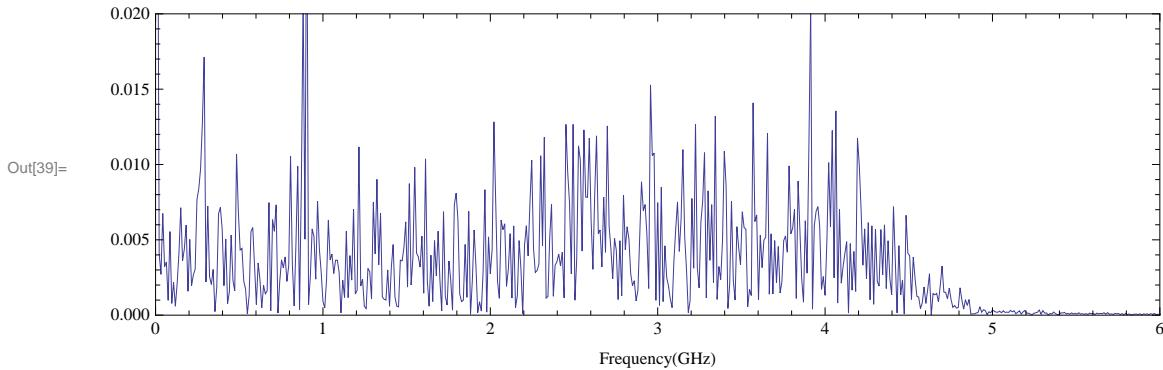
This has zero frequency in element 1. The 7693- th element corresponds to 1/2 the sampling frequency. After that aliasing takes over and the frequency heads back to zero.
