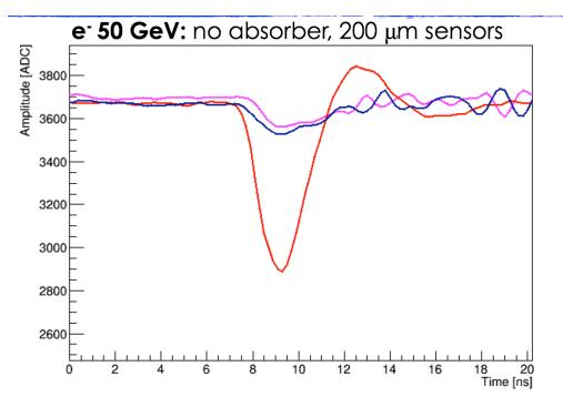
Above is a scope trace of HGC sensors for 1 MIP (not the nice trigger pulse but the 2 little pulses) from H2 this past month.
