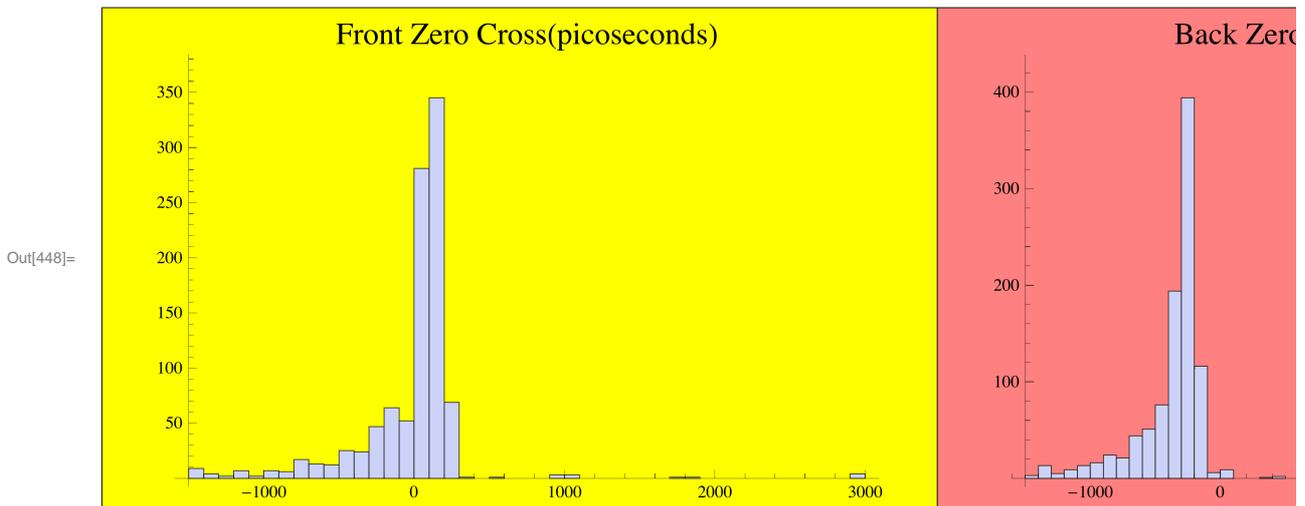
Deal with 9 cases out of 1000 where Roots of Interpolation function were not found for waveform. These were cases where scope triggered early and the roots are far from the initial search region.
