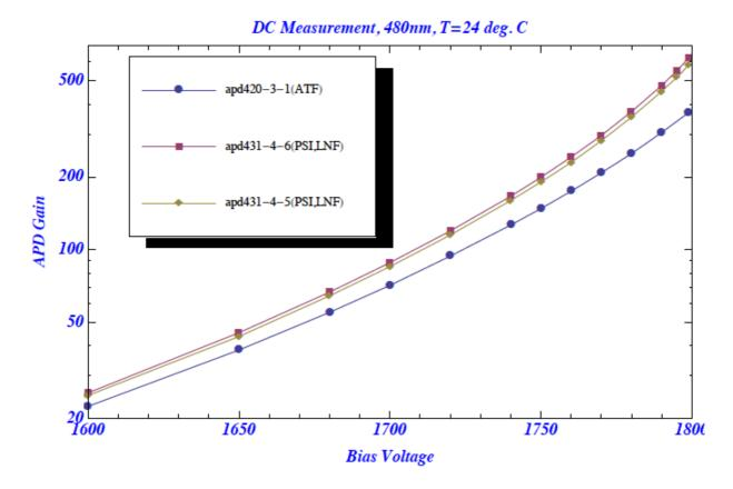
Uncertainties on expected pulse amplitude: 70 e - h/micron is taken from paper of Meroli et al.40 Micron is given by Dick Farrell as effective thickness of high field region. From the above Gain curve, the expected gain at 1795 V is in range~320 to 520 but private communication from Dick Farrel says one device (464 - 6 - 1) would correspond to higher gain curve above.
