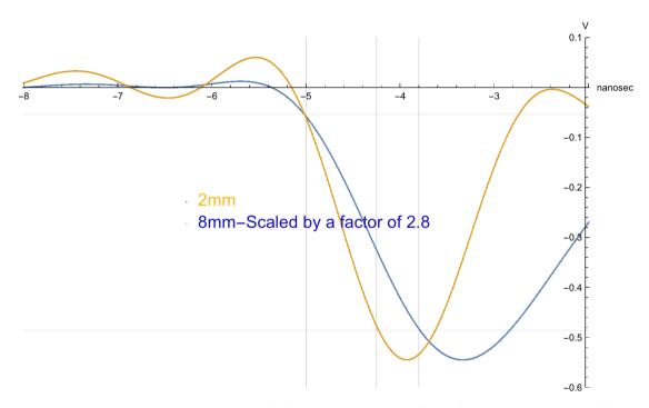
The Above waveforms were taken using the Wenteq amplifier (Freq. Response 10 - 1000 MHz and gain of 50 db) and the full scope bandwidth (4 GHz). They clearly show that the peak amplitude with 8 x8 mm APD is a factor of 2.8 lower than for the 2 x2 mm APD. They also show a deterioration of risetime (10 - 90 %) from 0.75 nsec to 1.2 nsec.
