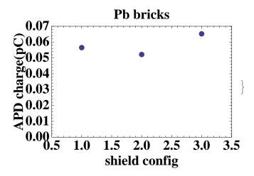
Let's consider the unshielded configuration with  $10^9$  e/pulse. It is 0.057 pC in a volume of  $64 \text{ mm}^2$  by  $60 \mu\text{m}$  depletion depth.
