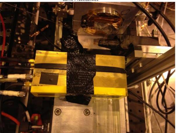
The detector housings locate on the jig alignment plate as shown above. To the left you see the relevant connectors (Vcc=3.4V, HV bias, Signal out). The "test pulse" input we don't use. The output goes to an external 13 dB additional amplifier using 5V power.
