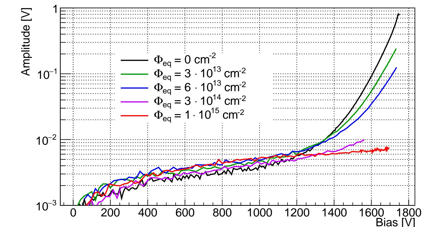
The irradiation increases the bulk generation current and reduces the gain of the detectors
