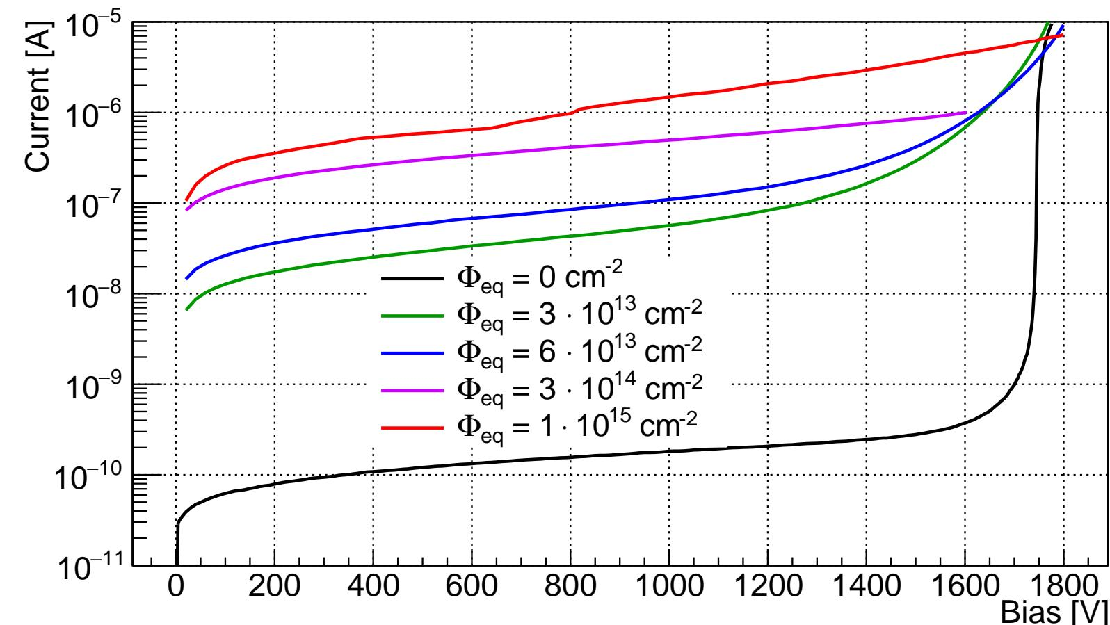
**Left:** current-voltage curves measured at  $-20^\circ\text{C}$
