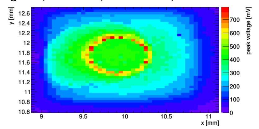
Red TCT signal peak amplitude map at -20°C and 1700V
