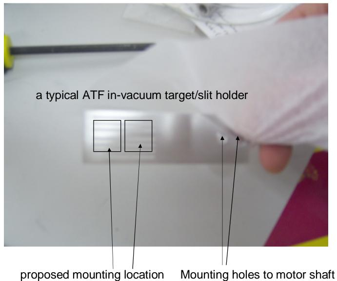
proposed mounting location Mounting holes to motor of Be & Cu targets
